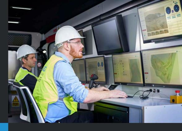
As vehicles detect obstacles, they alert the vehicle management system preventing others from facing the same issue. Once an obstacle is flagged, the vehicle management system generates a new route, or an operator can remotely access and assess the situation.
