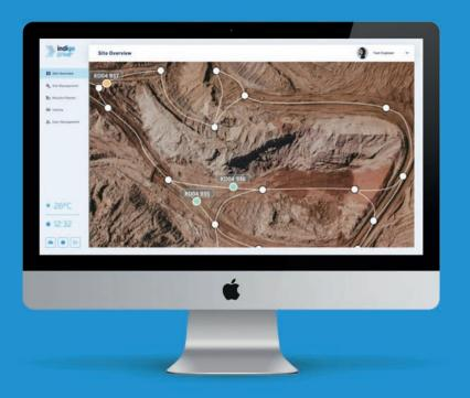
As vehicles detect obstacles, they alert the vehicle management system preventing others from facing the same issue. Once an obstacle is flagged, the vehicle management system generates a new route, or an operator can remotely access and assess the situation.
